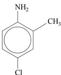
**Figure 1. 4-Chloro-2-Methylaniline Structure**
